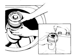
Clean dispenser after each use with warm water. To remove the dispenser, pull up on the top portion of the agitator. Clean by holding under faucet. Replace after cleaning.
